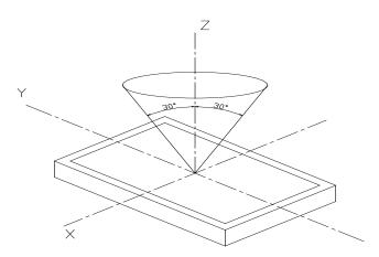
Inspection should be performed within angle  $\varphi$  ( $\varphi$  is usually 30°) from Z axis to each X and Y. Inspection distance in any direction within  $\varphi$  must be kept 30±5cm from the display surface.
