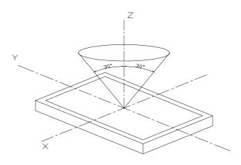
Inspection should be performed within angle ( is usually 30°) from Z axis to each X and Y.
